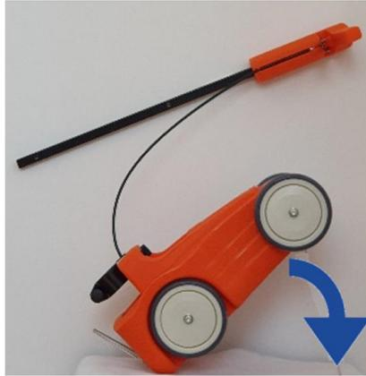
2- Swing the trolley back on its 4 wheels and the handle-bar onto the top side of the DRIVER™ with the handle facing backwards.
