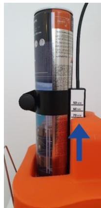
10- Set-up the line width by adjusting the height of the aerosol holder with the button-screw on the back of the sliding bar.
