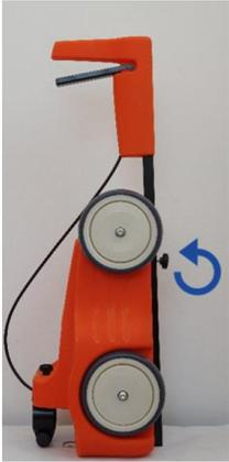
1- Unlock the screw on the back and keep it in the hand.
