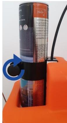
9- Tighten firmly the button-screw of the aerosol holder collar.
