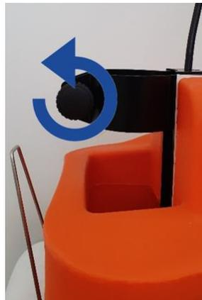
7- Unscrew the aerosol collar holder to ease the insertion of the paint can.
